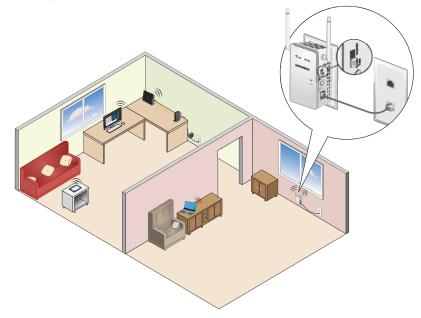
Figure 5. Extender as an access point
